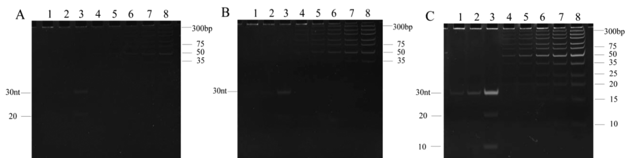
Figure 5. Fluorescence staining of nucleic acids in polyacrylamide gels by (A) TPE2, (B) TPE1, and (C) TPE3. Oligonucleotide size marker (X10, X20, and X30) with equal nanogram amounts of each oligonucleotide were loaded in lanes 1 to 3. Lane 1, 10 ng; lane 2, 20 ng; lane 3, 40 ng per band; ultra low range dsDNA ladder (10, 15, 20, 25, 35, 50, 75, 100, 150, 200, and 300 bases) were loaded in lanes 4 to 8. Lane 4, 1 ng; lane 5, 2 ng; lane 6, 4 ng; lane 7, 6 ng; lane 8, 12 ng per band at 300 bp. Concentration of dyes: 5 \mu\text{M} . Staining time: 30 min.
